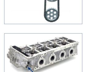
**On a limited number of vehicles**, this variation in length of the threaded shaft will require the housing on the head to be modified. This modification will be necessary in order to be able to correctly fit the tensioner.
